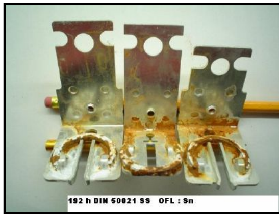
Figure 5 – Results of Salt Spray testing on silver plated copper NH contacts
